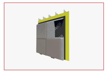
**Z CHANNEL OVER EXTERIOR BATT INSTALLATION**
